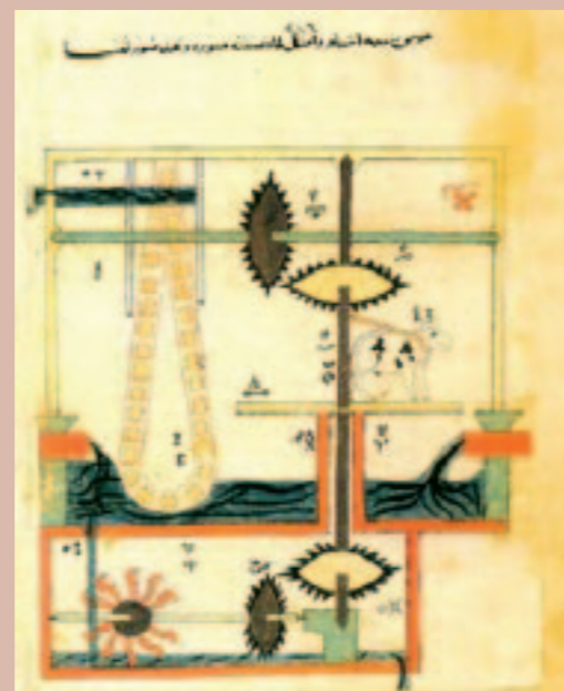
Al-Jazari's hydropowered saqiya chain pump device
